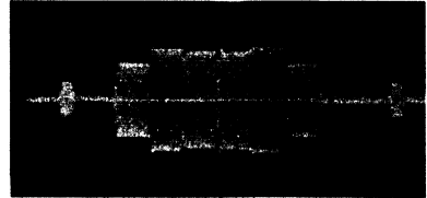
Fig. 21(b) - CA3071 terminal No. 6, amplifier No. 1 chroma output 2.3 V_{p-p} ; one horizontal line for 1.25 V_{p-p} chroma input
